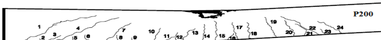
Figure 5. Crack patterns and flexural shear failure of Specimen P200.
